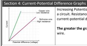
Increasing Potential Difference allows a greater Current to flow around a circuit. Resistance of a wire can be determined from plotting a current-potential difference graph for different wires.
