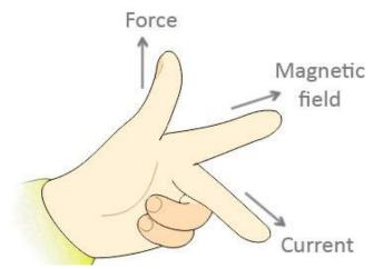
Align fingers to the field and the direction of the current to work out the way the wire moves.
